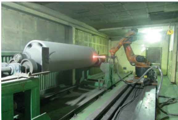
HP/HVOF Robotic Coating on Sink Roll
